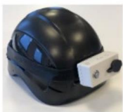
Figure 1. SmartHelmets and Bluetooth beacons
